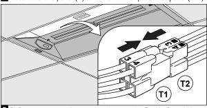
Before connecting the mains make sure the EvoKit SpaceWise is connected to the Evokit with the two halfs of the 4-pin connector.
