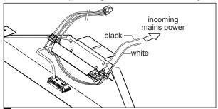
**6** Connect black and white wire from SpaceWise controller to incoming mains power. (A luminaire power disconnect can be added as necessary to these leads to meet any code requirements.)
