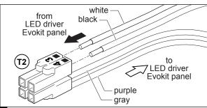
2 Insert purple wire from 4-pin connector (T2) to purple connector on LED driver on main panel. Insert gray wire to gray connector on LED driver. Insert white wire from LED driver to position 3 on connector and the black wire to position 4.
