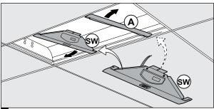
Install one side panel (A) and one EvoKit SpaceWise panel (SW)
